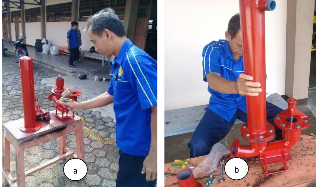
Gambar 3. (a) dan coating anti karat, (b) Set-up Pompa Hidram
