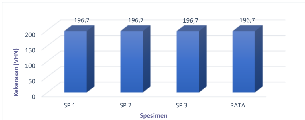
Gambar 4. Nilai Kekerasan Material Quenching berpendingin Dromus
